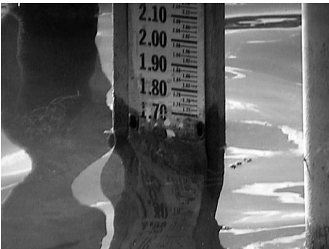
Figure 2. A typical lake level staff gage.
