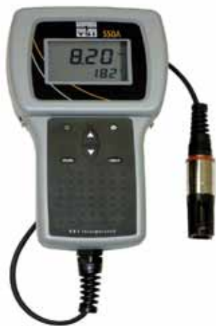
Figure 5. Portable dissolved oxygen and temperature meter with submersible probe as used in the Indiana Clean Lakes Program.
