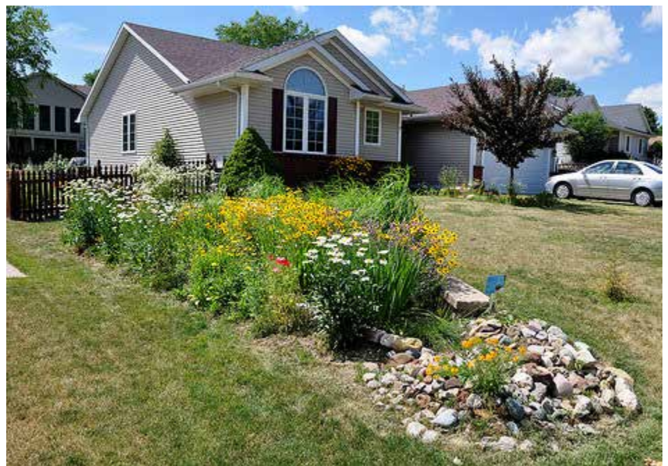
Figure 8. Rain gardens are depressed areas planted with perennial flowers and native vegetation that are meant to infiltrate rainwater. Rain gardens can be planted in yards or curb strips to provide plant diversity and living roots and ultimately improved water infiltration.
