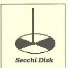
the experimental procedure for measuring transparency and today, the disk bears his name—the Secchi disk.
